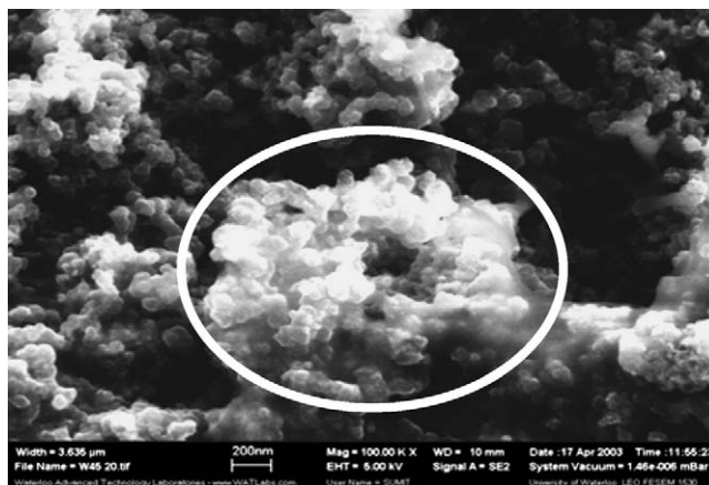
Fig. 5. Scanning electron micrograph of Nafion TM cluster (highlighted circle); resolution \times 100,000 .
